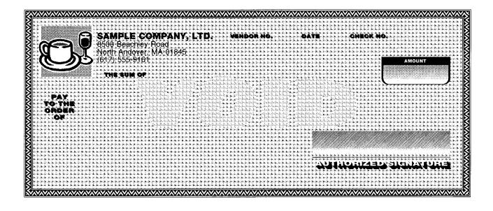
Figure 8a – Security document design with a combination of conventional halftone dots and custom halftone dots ("logodots").
