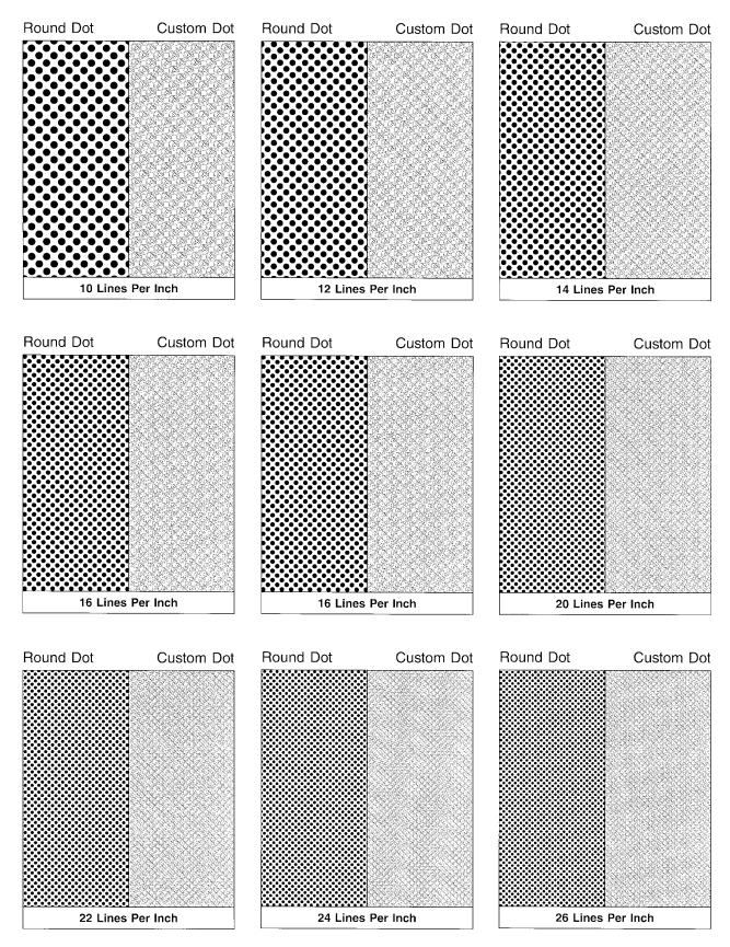
Figure 5a – Side-by-side examples of conventional halftone dots and custom halftone dot ("logodots") screens with 40% density at several line frequencies.
