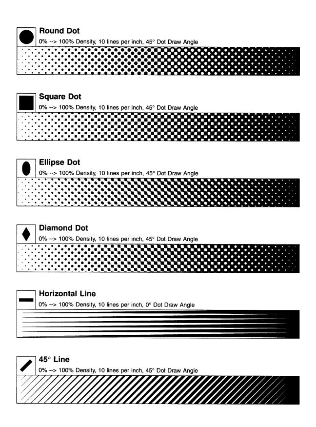
Figure 1 – Examples of conventional halftone dot and line screens.
