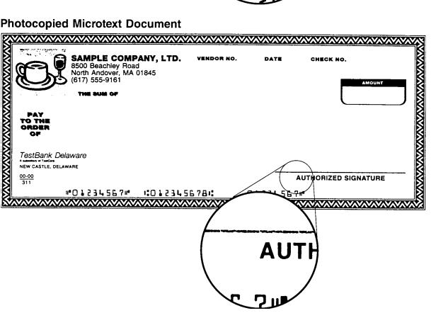
Figure 3 – Enlarged examples of microtext before and after a photocopy.
